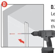
**D.1**Level against the wall, mark and drill the holes
