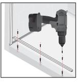
**D.3**Mount U-channel with desired fasteners. Fasteners anchored into ceiling, if required for the application, must hit solid
