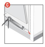
**C.1**Use silicone sealant to seal inside of miter joint prior to installing glass panel
