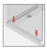
**A.3**Then drop into bottom u-channel with setting blocks.
