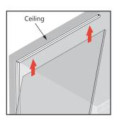
**A.2**Carefully slide panel into top u-channel
