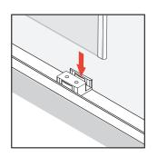
**B.2** When attaching glass door to rollers gently align into panel guide
