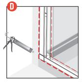
Apply silicone sealant to the interior and exterior frame to prevent water leakage
