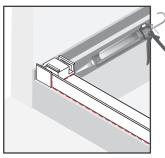
Insert bottom sill into side rail shoe and silicone into place If curb/base is out of level more than 1/4", shim as required for proper adjustment
