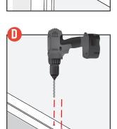
**D.1** Drill holes through the sill plate only, not into the shower curb
