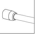
Make sure that the flat side of rod mount faces out to allow glass panel door to fully operate.
