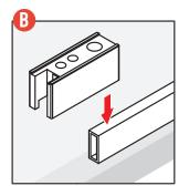
**B.1** Insert rollers on to rails as pictured before attaching to glass doors.
