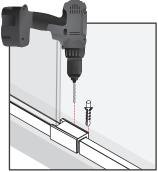
**A.2** Drill holes and insert anchors for screws
