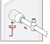
Tighten set screws and secure with loc-tite once rod is in desired position
