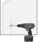
Drill holes. Note: Hole should be 3/8" (10mm) in diameter. The mounting bracket will give you about a1/4" play up or down for the rod
