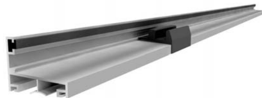
SILL W/ FLOOR GUIDE (USE A SILL WHEN THERE IS NO SLOPED CURB)
